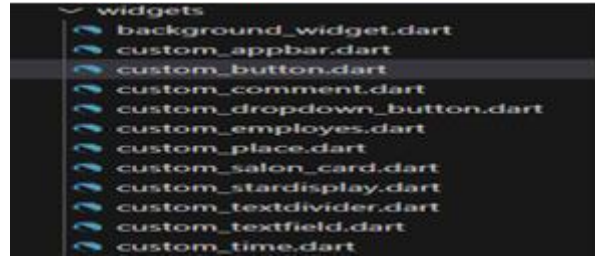
Fig. 2 Widgets are the basic building blocks of creating the user interface. Each widget is a Dart class that performs a specific function and represents UI elements that are displayed or interacted with. For example, it has made it easier to create a dynamic application by creating different widgets that can represent a button, text box, image or a list item.
